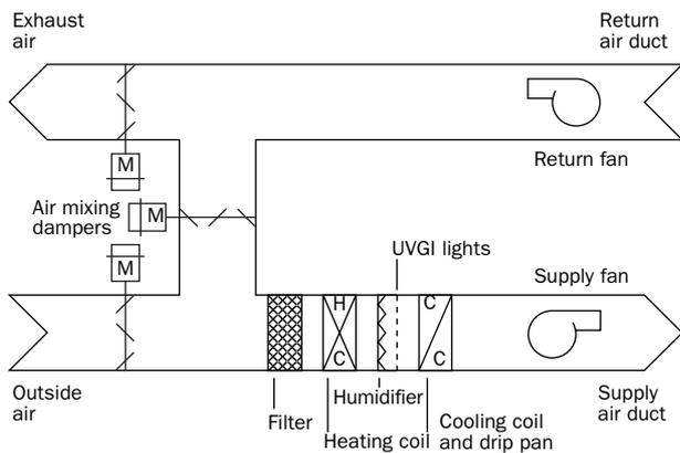
Figure 1: Schematic diagram of a typical HVAC system
